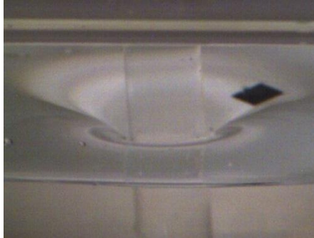
Figure 5.42: Picture of a 1 mm part at an equilibrium distance near a 2 mm diameter hydrophobic rod.
