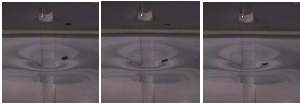
Figure 5.22: Close view of micropart on hexadecane-water interface.
